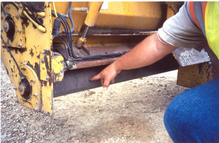
Figure 7-33. Discharge Roller on Aggregate Spreader.
