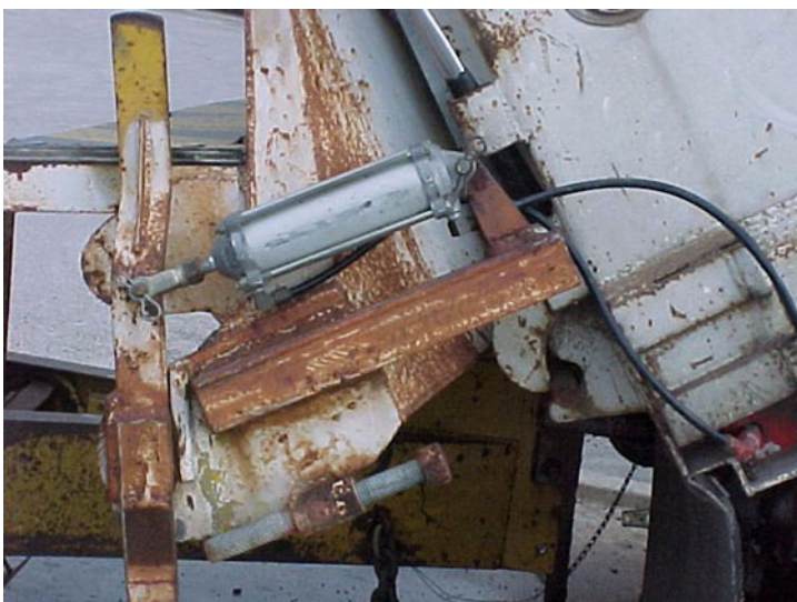
Figure 7-37. Air Cylinder to Open/Close Spreader
