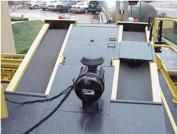
Figure 7-30. Belt Conveyors on Aggregate Spreader.
