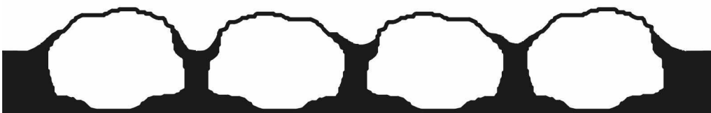
Figure 8-7. Decrease in Volume after Emulsion Has Cured.
