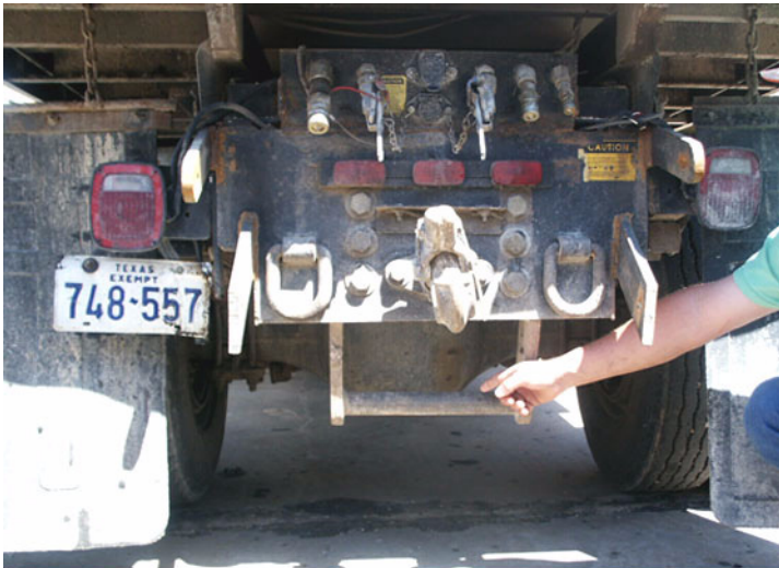
Figure 7-40. Truck Hitch to Connect to Aggregate Spreader.
