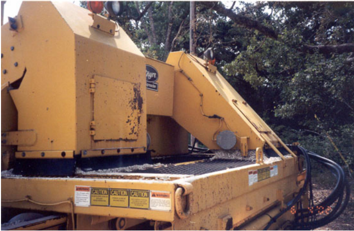
Figure 7-31. Discharge Hopper of Aggregate Spreader.
