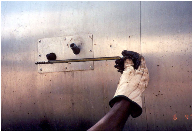
Figure 7-5. Thermometer Removed from Distributor Tank.
