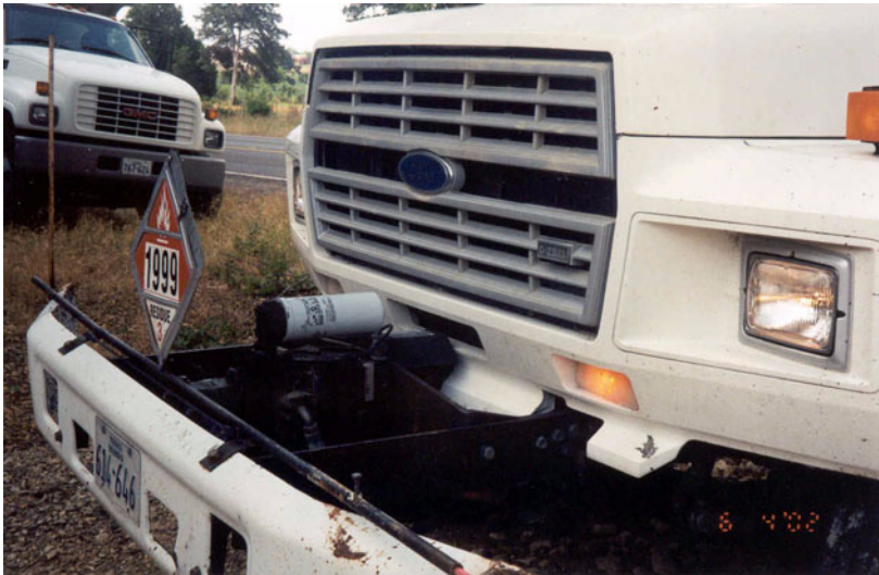
Figure 7-8. Hydrostatic Distributor Located at Front of Truck.
