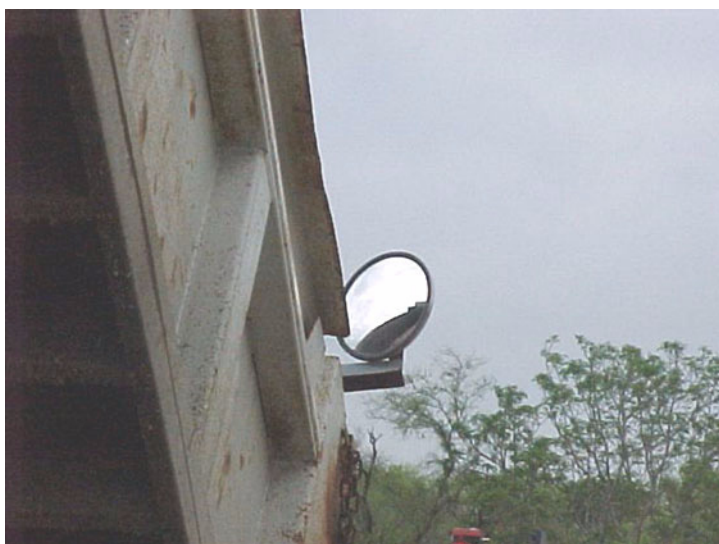
Figure 7-36. Mirror to View Rock in Truck and Rock Flow
