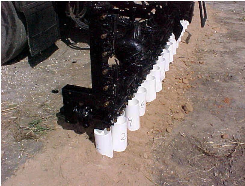
Figure 7-21. Calibration of Asphalt Distributor Spray Bar.
